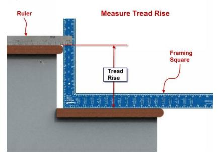
Step 2. Using 2 squares determine the exact nose to nose run of each tread, record on the worksheet.
