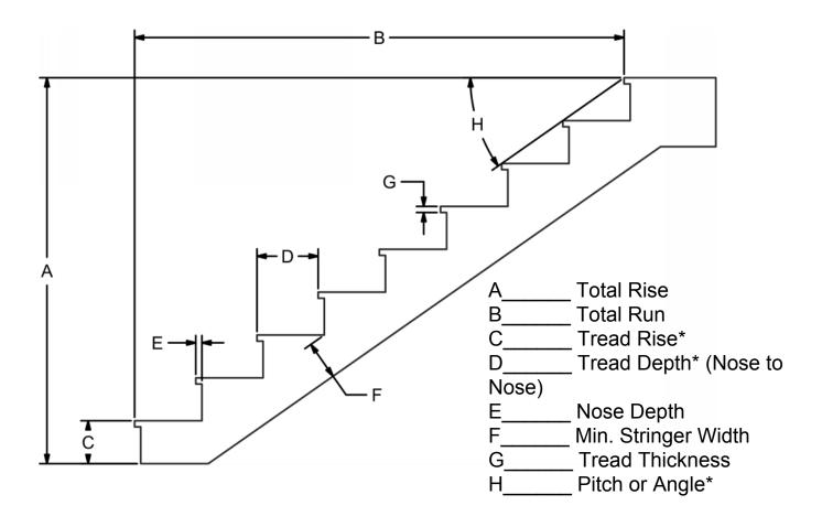
**Measurements:** Very carefully measure the stair and fill in this form. \*Measurement C,D and H are the most <u>critical</u> to ensure proper railing fit. See measuring guidelines on the next page for help.
