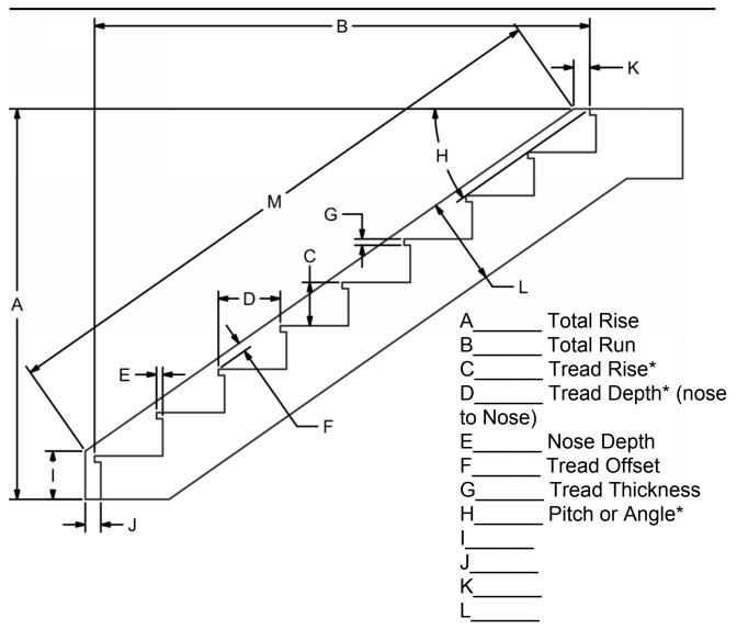
**Measurements:** Very carefully measure the stair and fill in this form. \*Measurement C,D and H are the most <u>critical</u> to ensure proper railing fit. See measuring guidelines on the next page for help.
